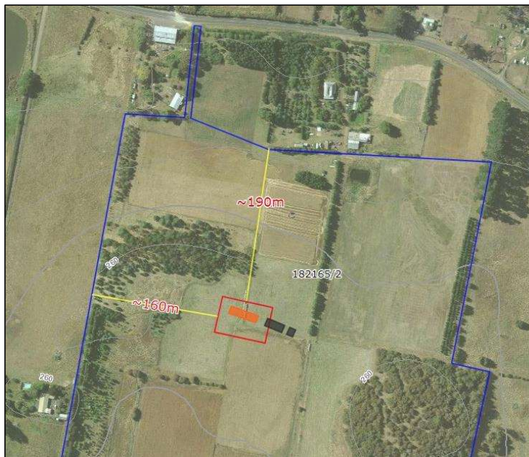
Figure 7. Setback distances (yellow lines) of proposed dwelling envelop (red outline) from title boundaries (blue lines). Setbacks greater than 200m have not been shown (Source: The LISTMap).
