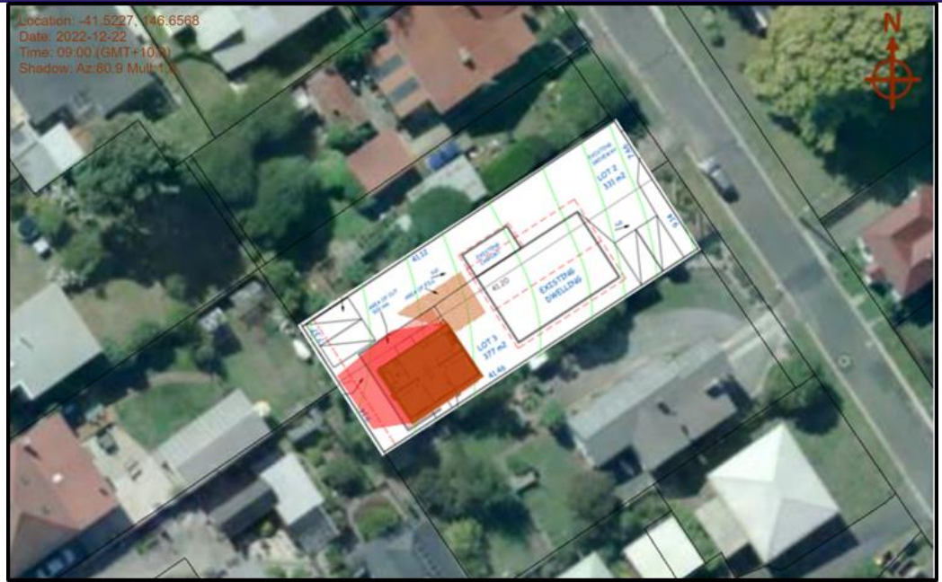
Figure 3: Shadow diagrams (not to scale) of the proposal at 9am on 22 nd December.
