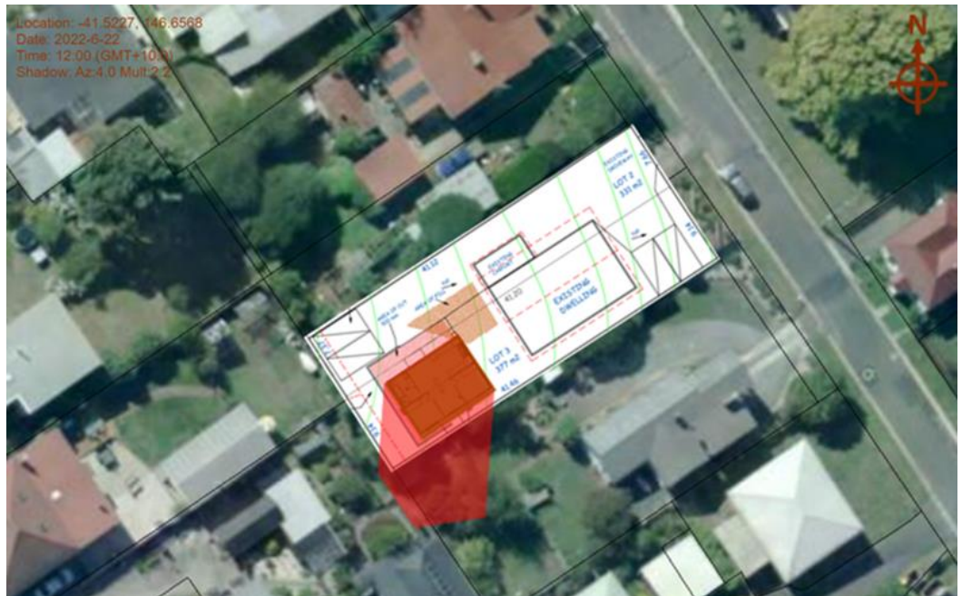
Figure 4: Shadow diagrams (not to scale) of the proposal at 12pm on 22 nd June.
