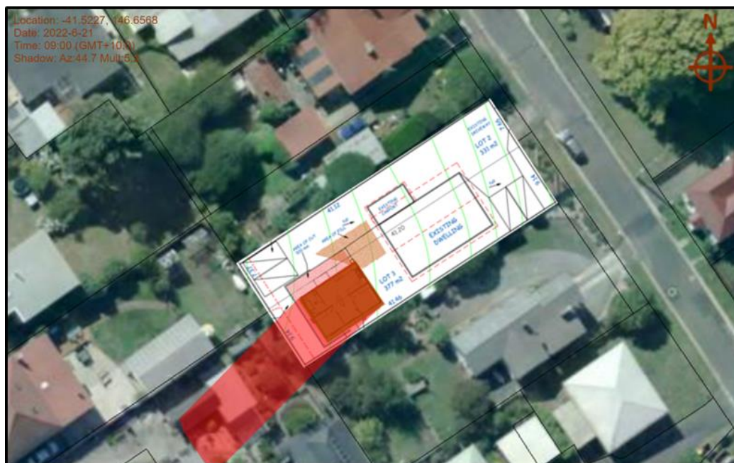
Figure 2: Shadow diagrams (not to scale) of the proposal at 9am on the 22 nd June.
