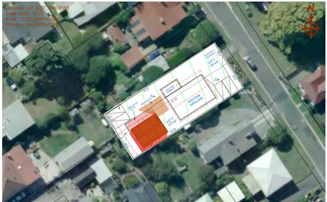
Figure 5: Shadow diagrams (not to scale) of the proposal at 12pm on 22 nd December.
