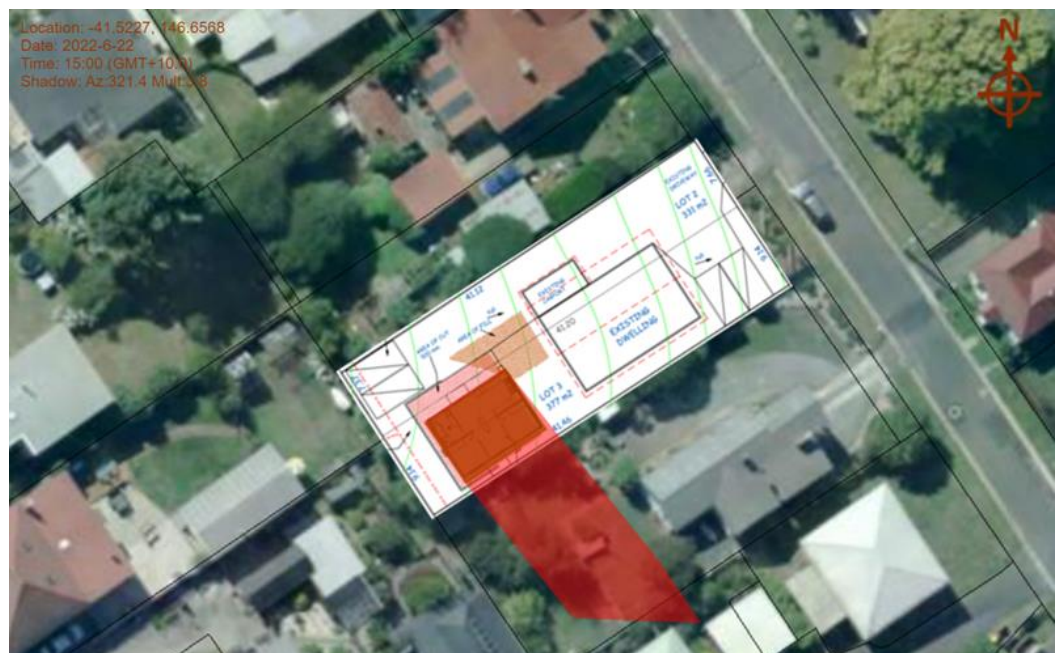
Figure 6: Shadow diagrams (not to scale) of the proposal at 3pm on 22 nd June.
