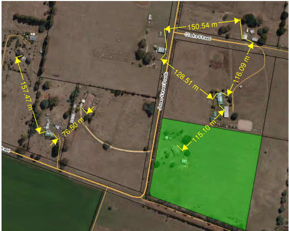
Figure 4 - separation distances between existing adjoining and adjacent building areas on lots to the north and west of the site.
