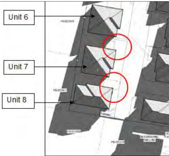
Figure 10: Shadow Plan at 9.00am. Private open space not in shadow circled in red.
