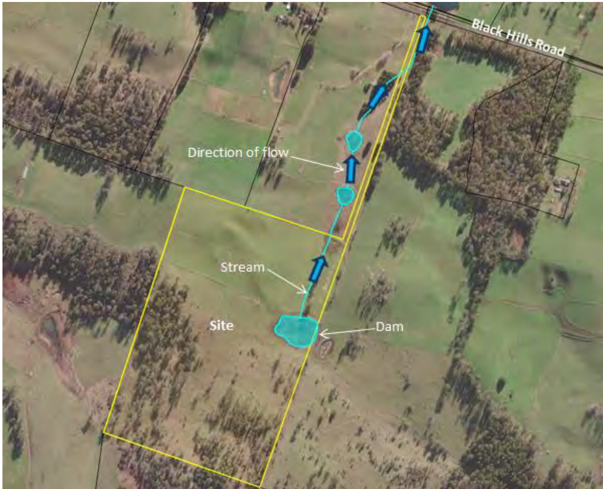
Figure 2 - Aerial image illustrating the location of the dam within the site and the spatial extent and flow direction of the stream.
