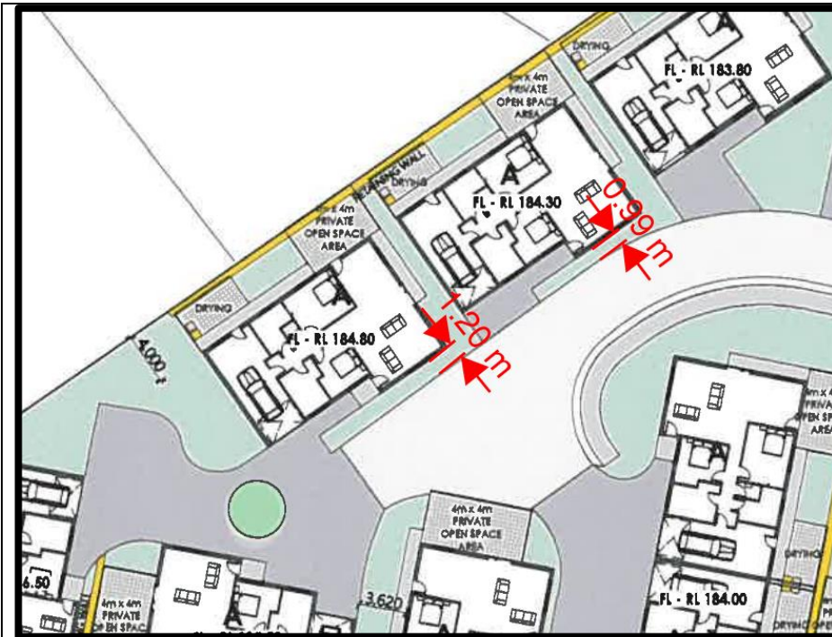
Figure 13: Showing the separation distance between Units 58 and 59 to the internal driveway.
