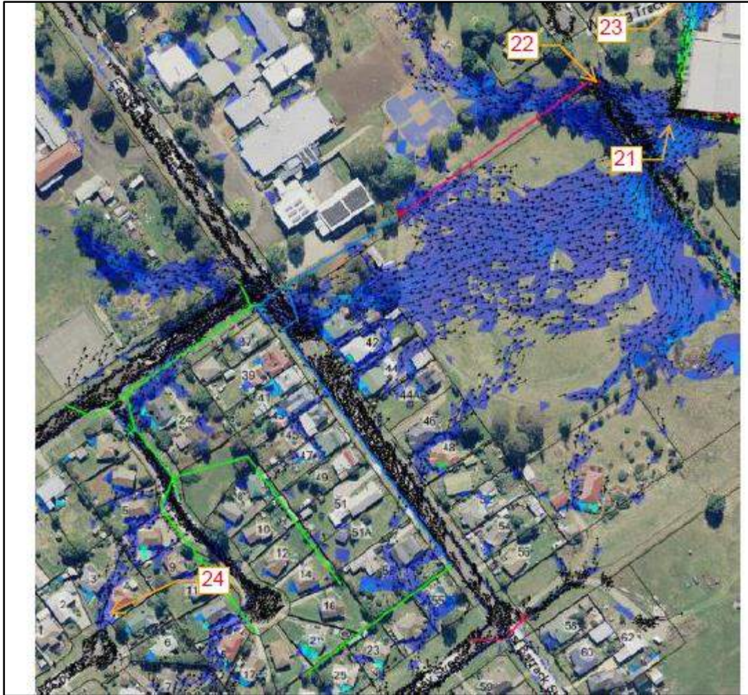
Figure 9. South Deloraine – Pultney Street Stormwater System 1% AEP.
