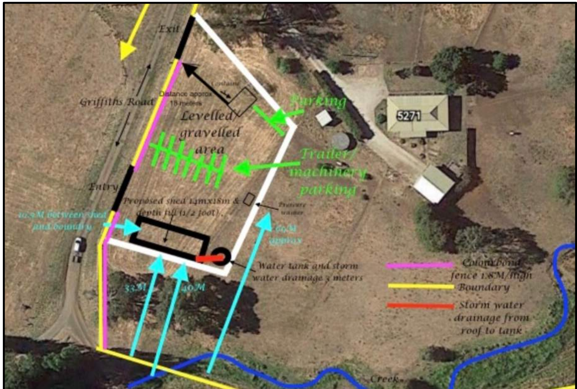
Figure 1: Site plan for the proposed Transport Depot. Refer to attachments for full site plan.
