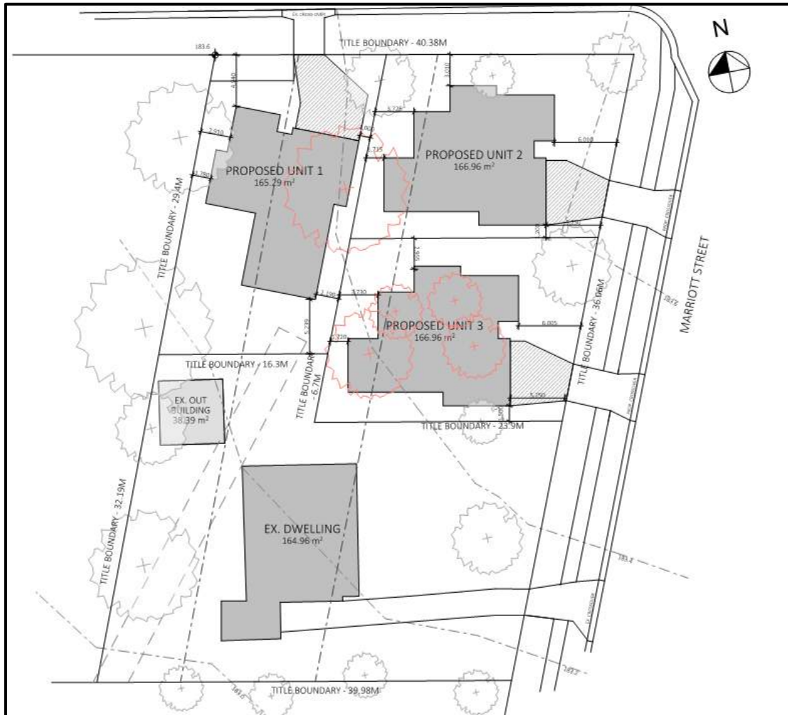
Figure 2: Site plan showing the existing dwelling, proposed new title boundary and location of three (3) units.
