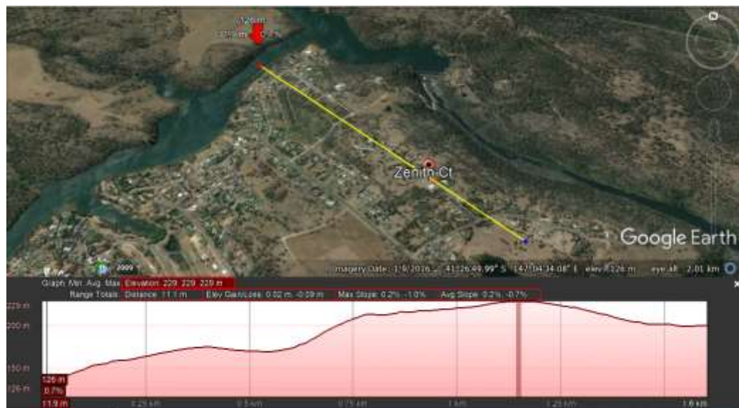
Figure 7: Cross-section of topography showing the elevation of the subject site between South Esk River and Canopus Drive (source: Google Earth Pro). The location of the subject site shown by the dark pink line indicating the highest elevated point in the landscape
