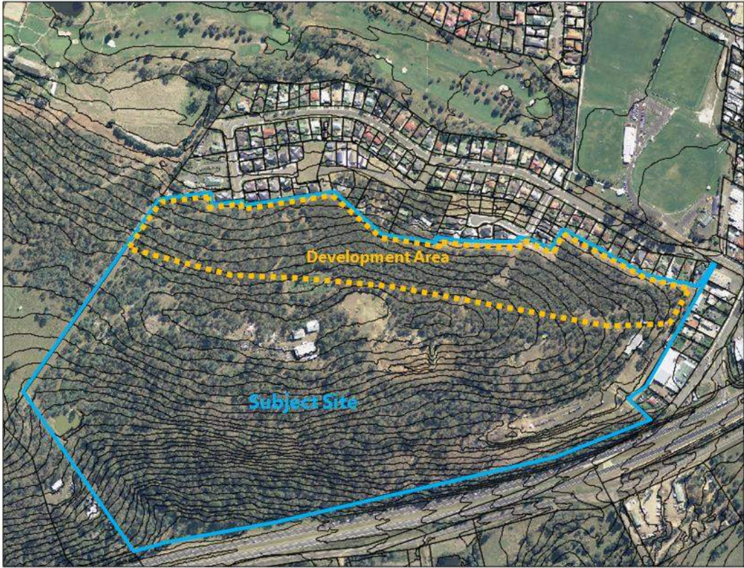
Figure 3 – Aerial photo of the subject site showing 2 metre contours and development area.
