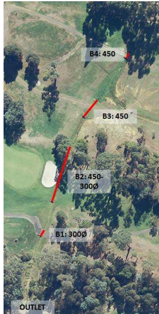
Figure 16. Western drain culverts
