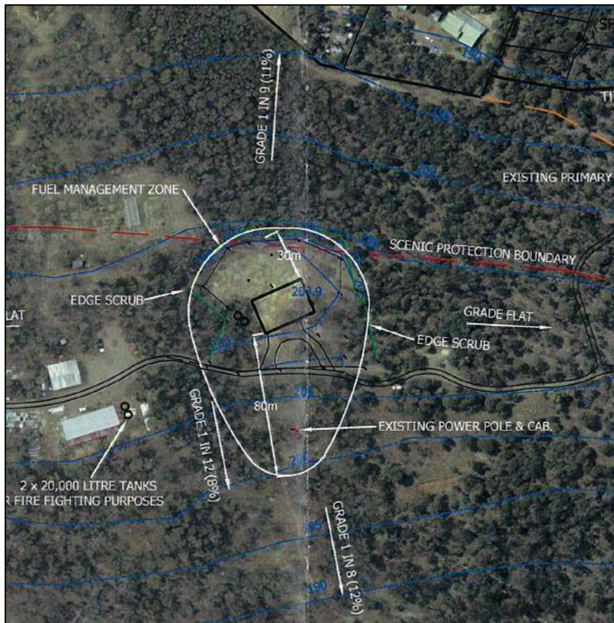
Figure 3 – Excerpt of Bushfire Hazard Management Area for the adjoining dwelling under construction.
