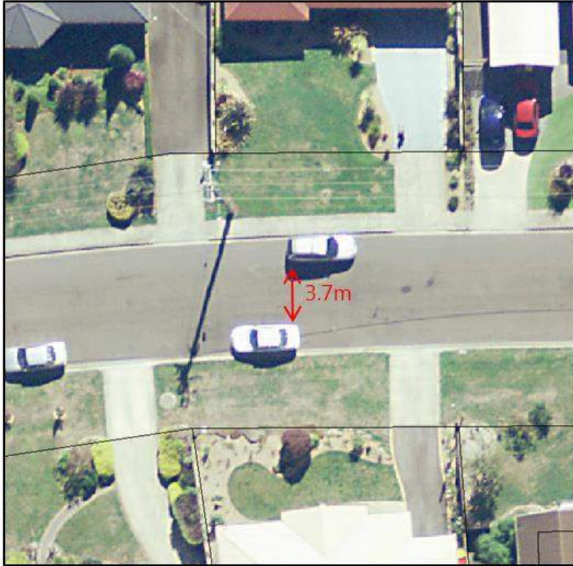
Figure 2 – Aerial photo view of constrained carriageway of Harley Parade when street parking occurs to either side.
