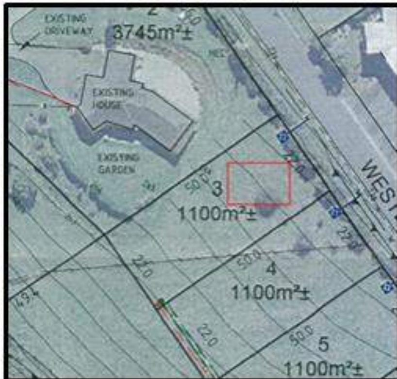
Photo 5: showing a red 10m x 15m building area for Lot 3.
