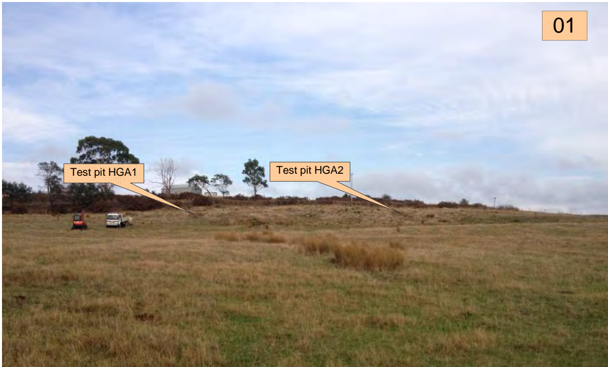
01. View SW towards Area A near Saunders Drive, 1 April 2015. Dolerite bedrock was exposed at shallow depth in both test pits. This area is low geotechnical risk.
