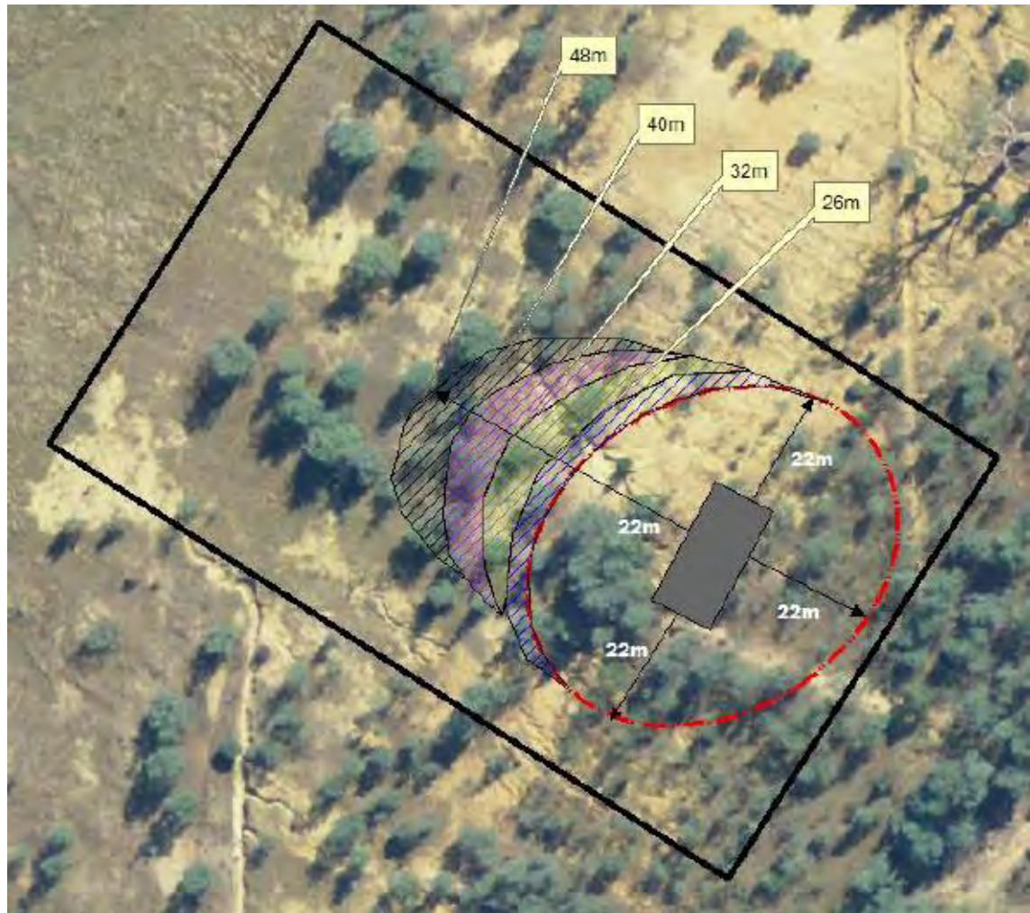
Figure 10 Hazard Management for dwellings to BAL 12.5, based on slope (Ground Proof Mapping , 2014)
