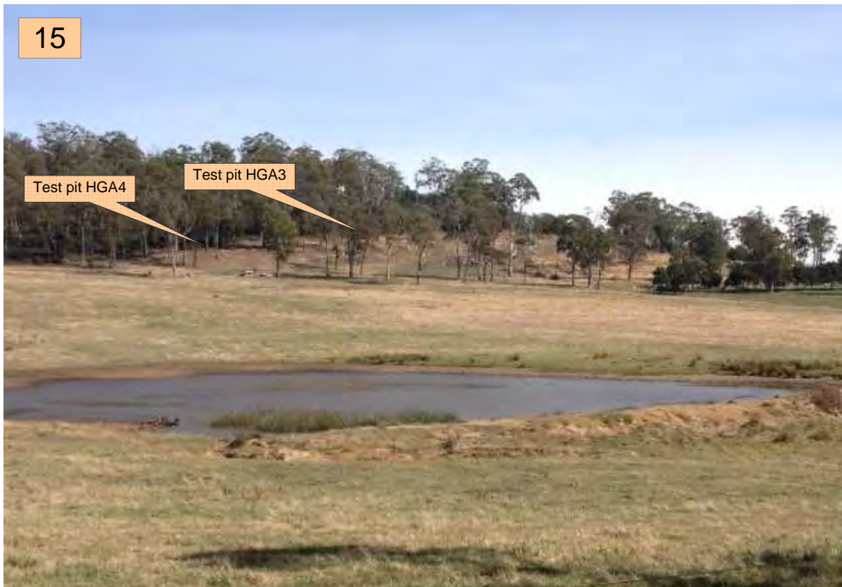
15. View SW towards Area C from Saunders Drive, 1 April 2015. Dolerite bedrock was exposed beneath sand at shallow depth in both test pits. This area is low geotechnical risk.
